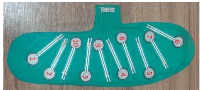
Fig.4. Sensor placement in insole shoe
