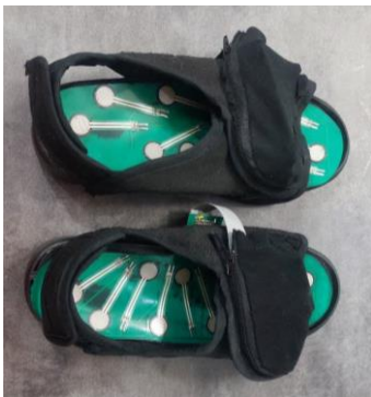
Fig. 3 (a). Overview of the designed shoe
