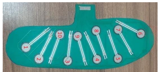
Fig.4. Sensor placement in insole shoe
