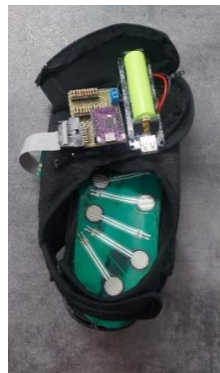
Fig. 3 (b). Positioning of the electronic board and control module
