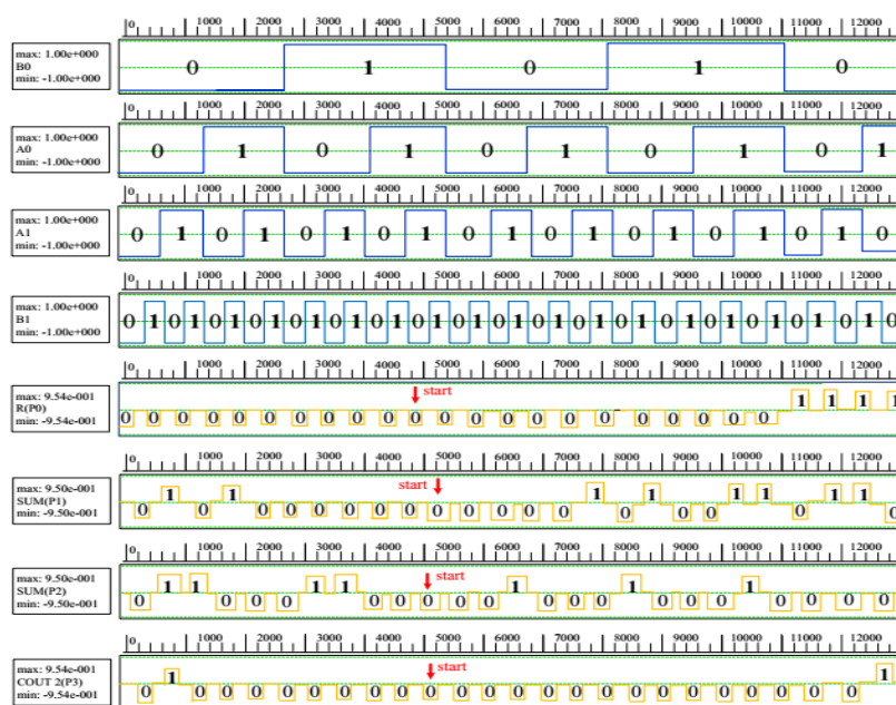
Fig. 25. The results of the 2 \times 2 multiplier circuit.
