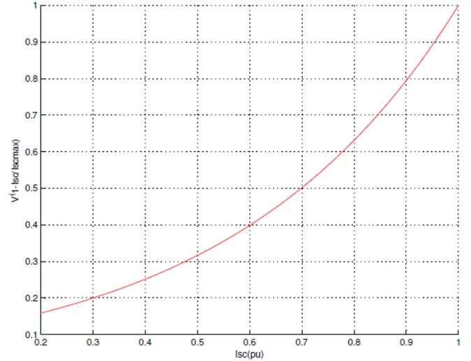
Fig. 4.  $K_d$  factor variation vs SCC intensity
