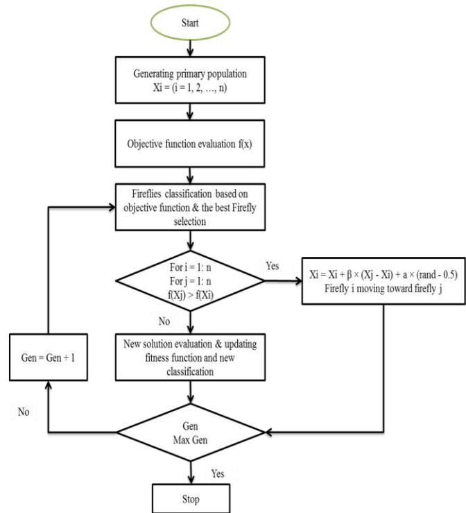
Fig. 2. The flowchart of FA operation process
