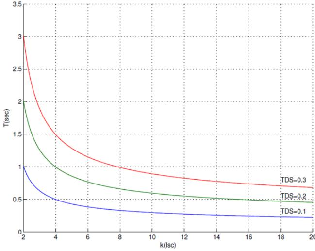
Fig. 3. OCR switching time for a specified SCC range
