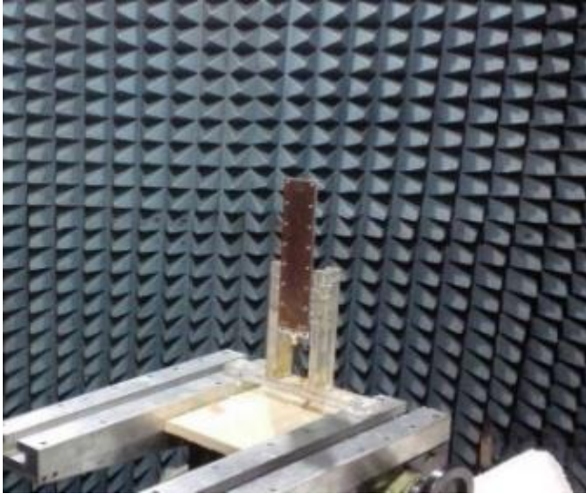
Fig. 5 The radiation pattern measurement in an anechoic chamber.
