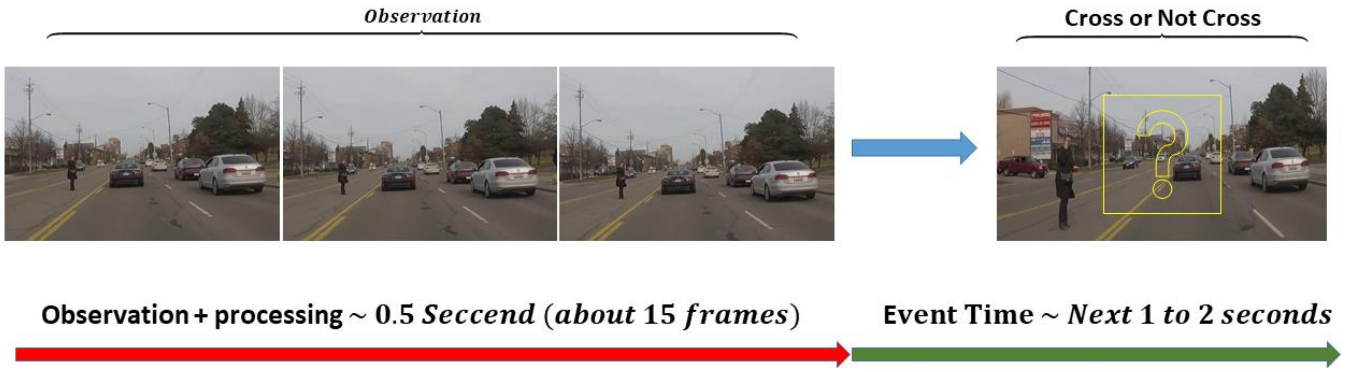
Fig. 1. The operation of predicting pedestrian crossing or not crossing the intersection. According to the sets of observed frames, this operation predicts the event of passing or not passing the pedestrian in the future so that the self-driving vehicle has enough time to react to the behavior of the pedestrian.
