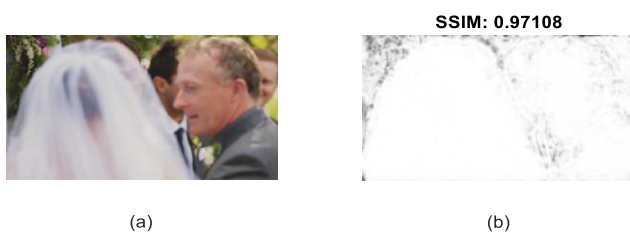
Fig. 8. SSIM map for a random frame sample (a) Improved frame using the proposed method (b) SSIM map of the same frame
