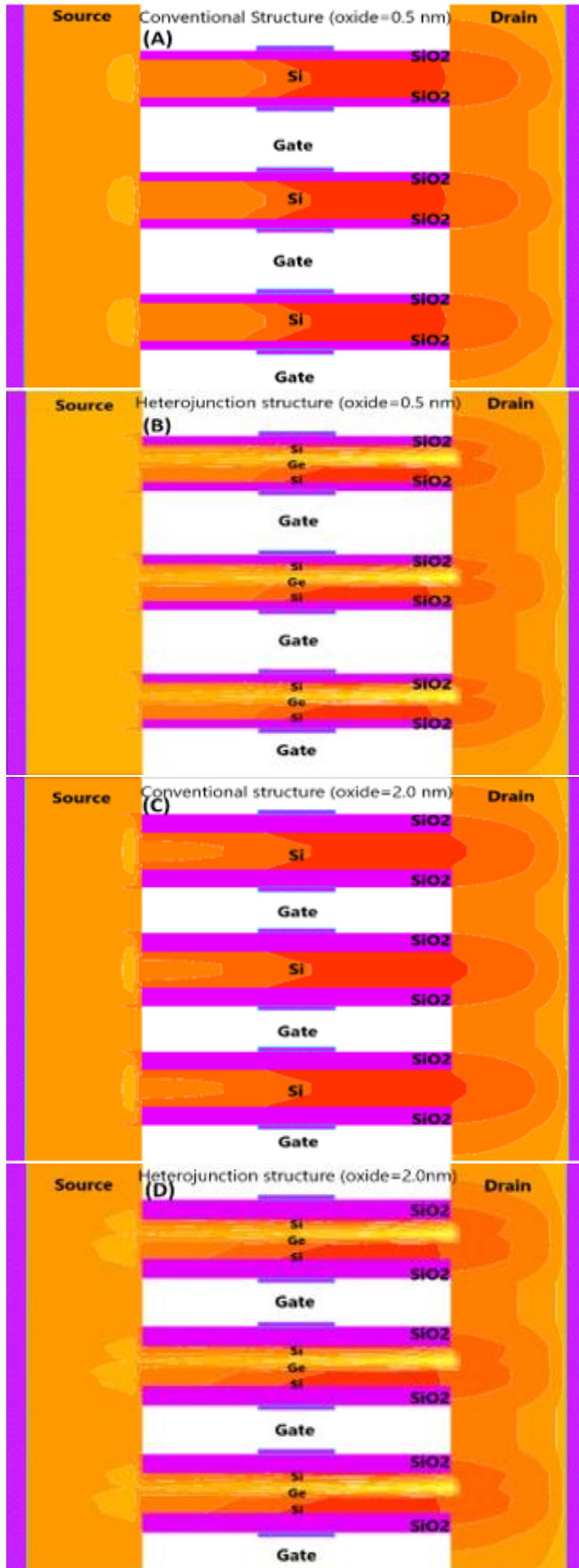
Fig. 5 (A-D): Electron densities varying with the same gate to source voltage for Heterojunction GAA NS FET and Conventional GAA NS FET with different oxides
