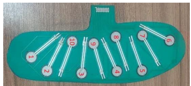
Fig.4. Sensor placement in insole shoe
